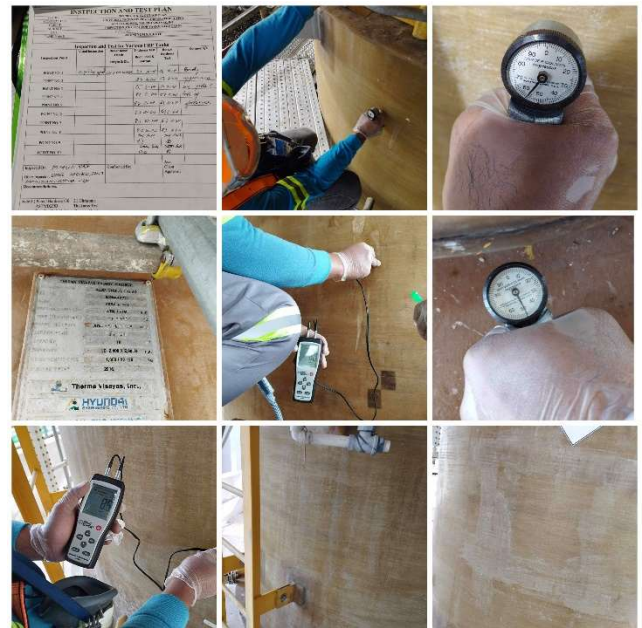
FRP Tank Hardness and Thickness Inspection
