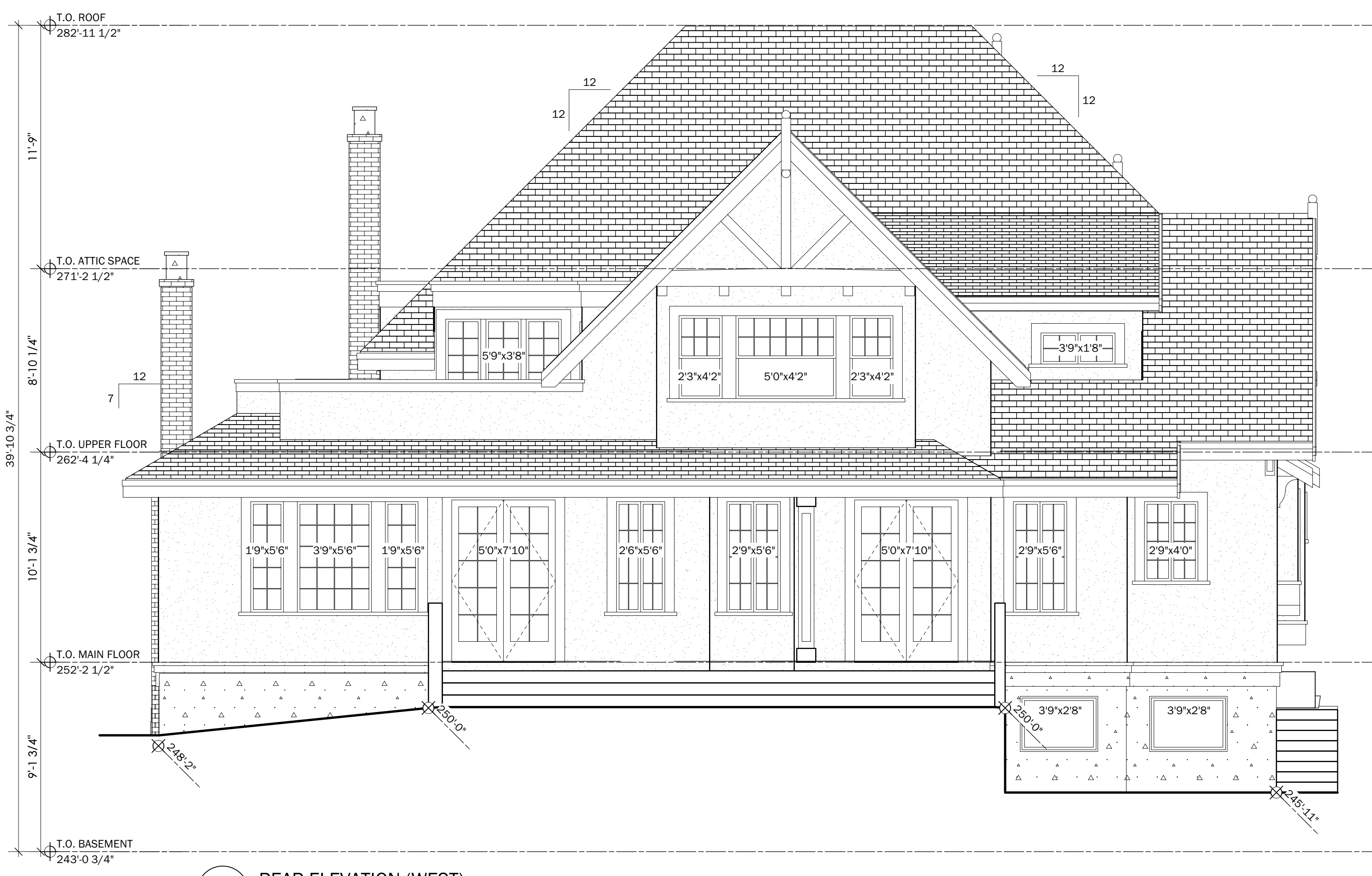
2 REAR ELEVATION (WEST) Scale: 1/4" = 1'-0"
