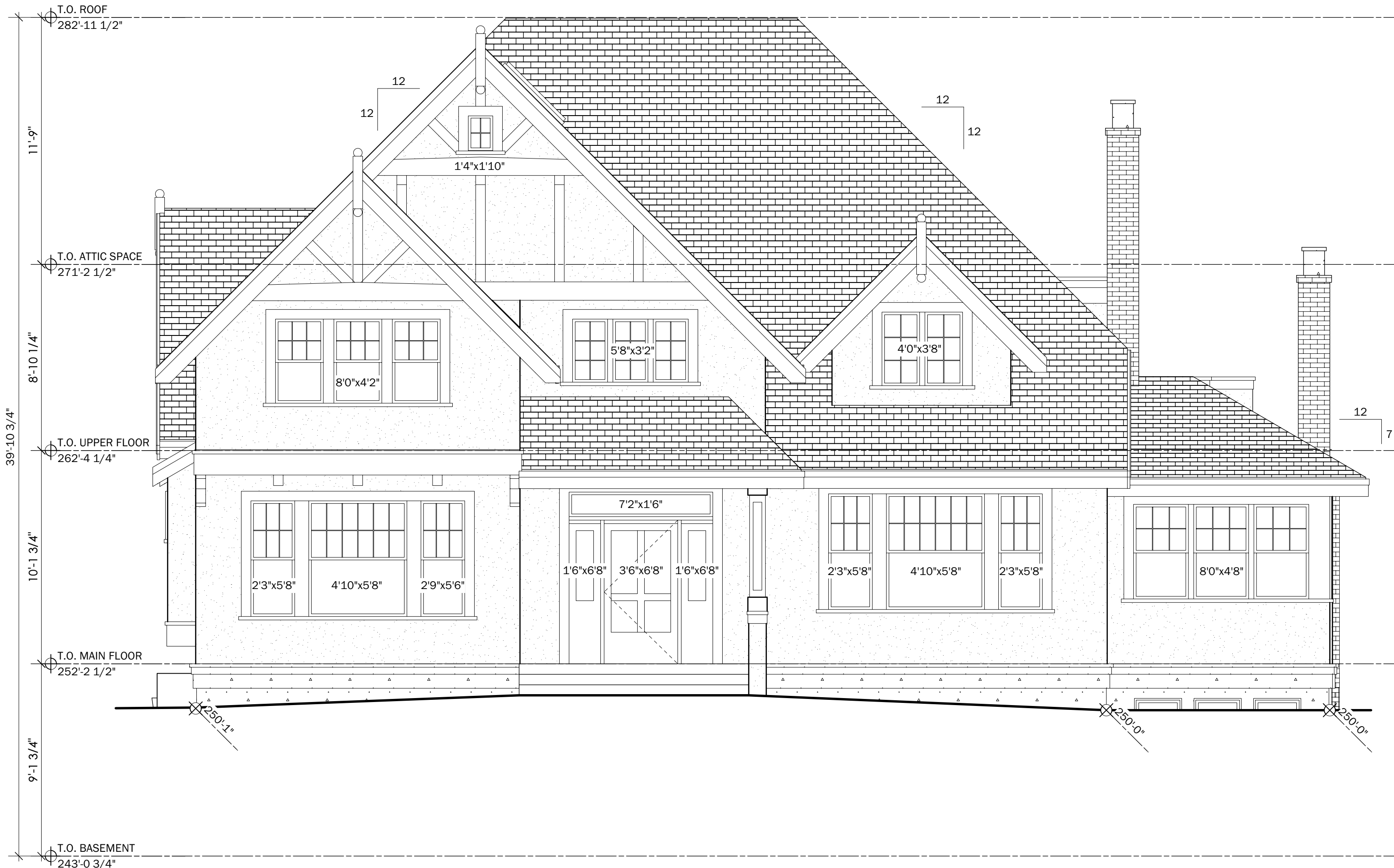
1 FRONT ELEVATION (EAST) Scale: 1/4" = 1'-0"
