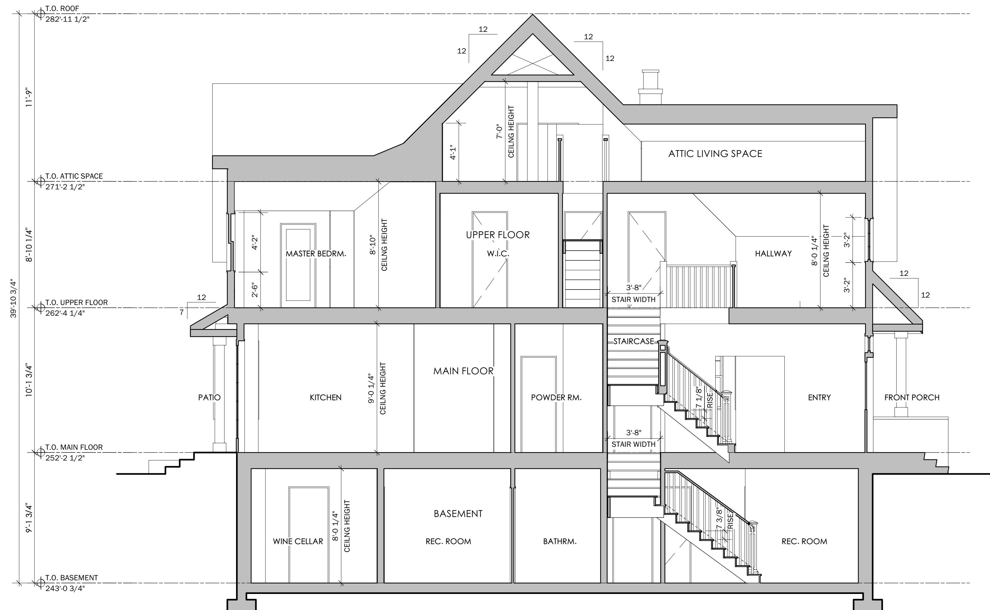
2 CROSS SECTION THRU ENTRY & STAIR Scale: 1/4" = 1'-0"
