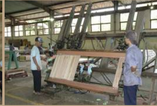
Assembly and hydraulic pressing with pressure indicator.
