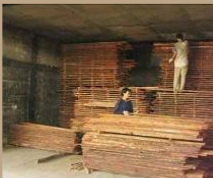
Kiln dry : 7 chambers up to 350m 3 , electronic panel, timber moisture content controlled regularly.
