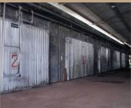
Kiln dry : 7 chambers up to 350m 3 , electronic panel, timber moisture content controlled regularly.
